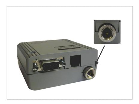
Figure 8. Antenna interface – FME jack
