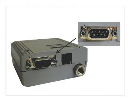
Figure 4. M terminal RS232 pin assignment (D-Sub9 female)
