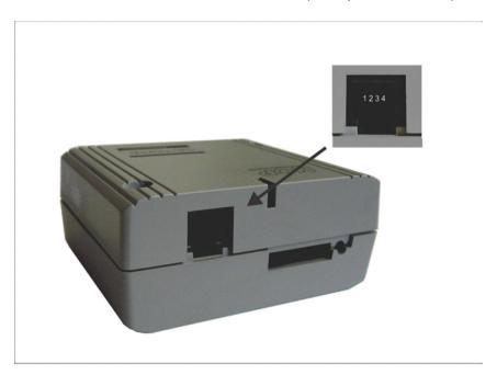
Figure 5. Audio interface connector
