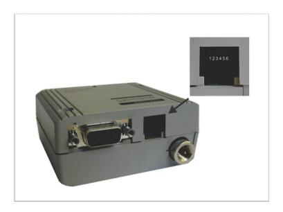
Figure 3. Power supply connector
